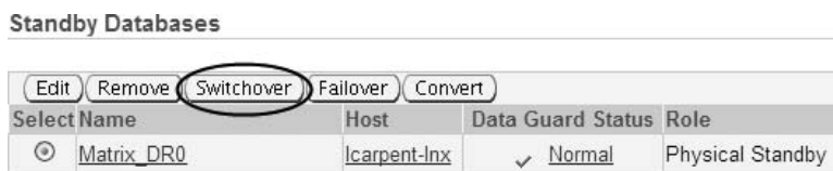
FIGURE 8-5. Using Grid Control to switchover
